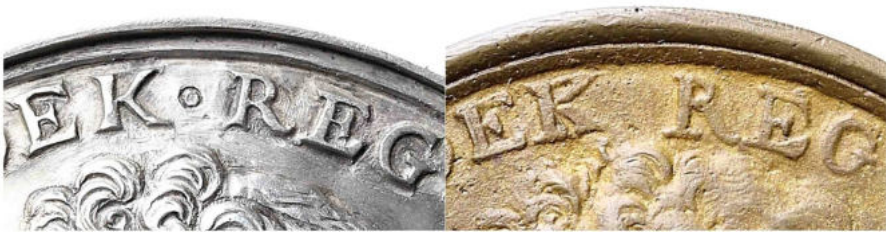
Fig. 4 – Detail of medal A1 (left) and B1 (right) showing the irregularities due to casting
