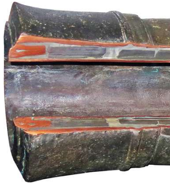
Picture 39 – Cross-section of the mouth of a cannon from the shipwreck of the Batavia , sunk in 1629 off the coast of Western Australia.
